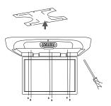
4. Flip the monitor screen down and tighten the monitor to the support bracket, using the supplied screws.
